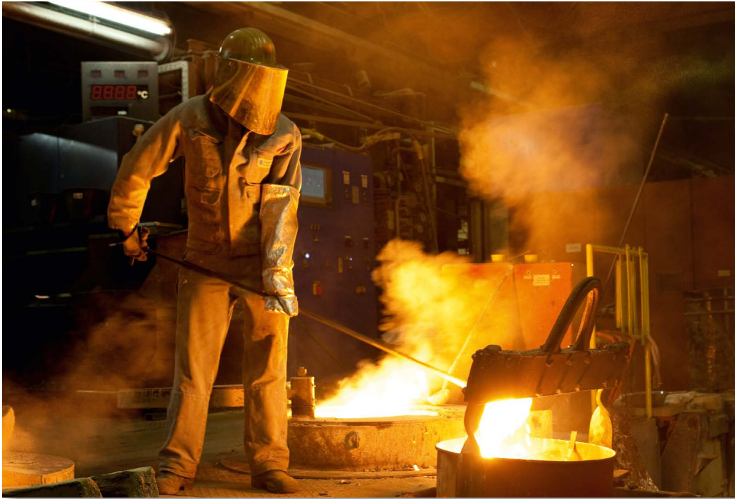
Deslagging of a stainless steel melt at a temperature of 1,600 degrees celsius
